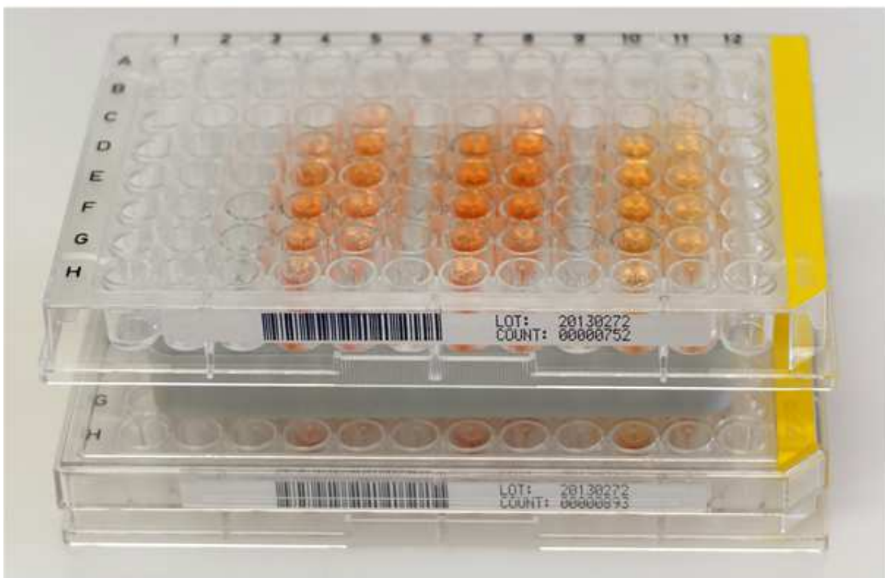
Figure 1: Alignment of 96-well plates below and above a Mini-Rayonex device with its lettering pointing upside and to the front. The multiplates were placed exactly in this way into the external incubator at 37.2 \pm 0.2 °C. The lower part of the figure represents the wells with seeded and exposed cells which have cleaved the tetrazolium dye due to their vitality and activity of mitochondrial dehydrogenases (orange coloured wells).
